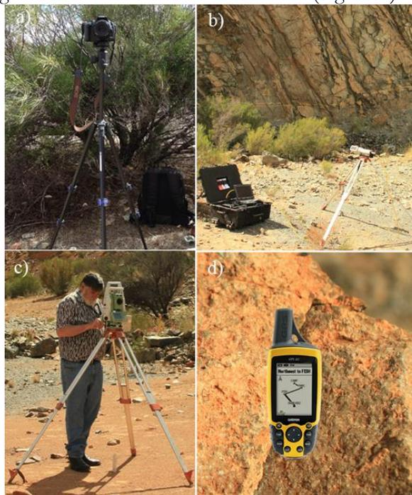
**Figure 1.** Field Equipment. (a) Canon EOS 350D digital camera; (b) MDL void laser scanner VS150; (c) Leica TS150 total station; (d) Garmin T60 hand-held GPS
